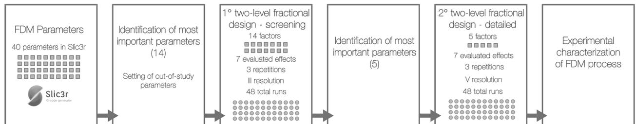
Fig. 1 Recommended FDM characterization procedure
