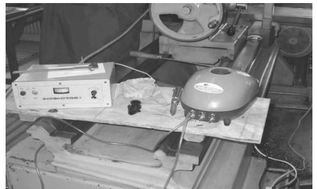
Fig. 4 Working assembly of the source of fair ionization
