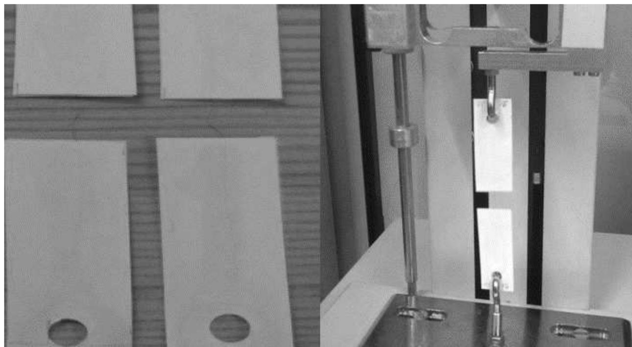
*Fig. 1 Scheme of biopolymer string testing*
