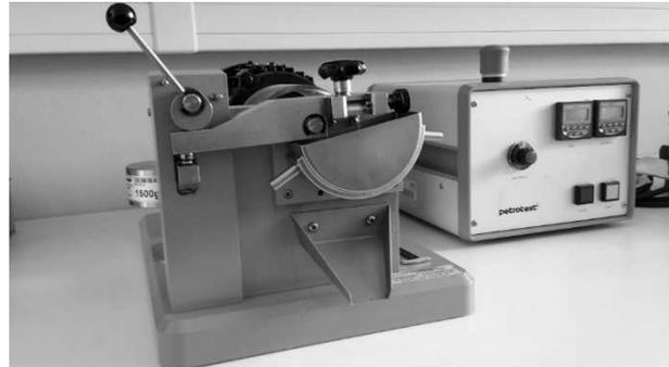
Fig. 1 Reichert Friction and Wear Tester.
