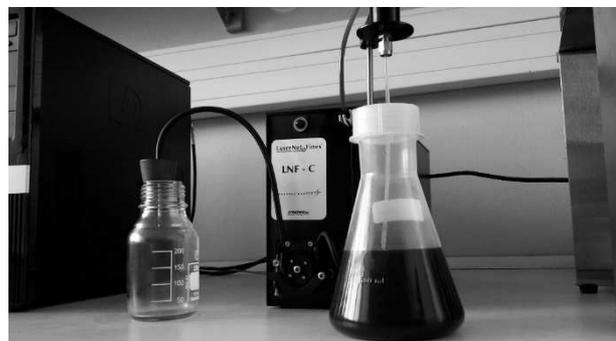
Fig. 2 Particle counter and shape classifier LaserNet Fines-C.
